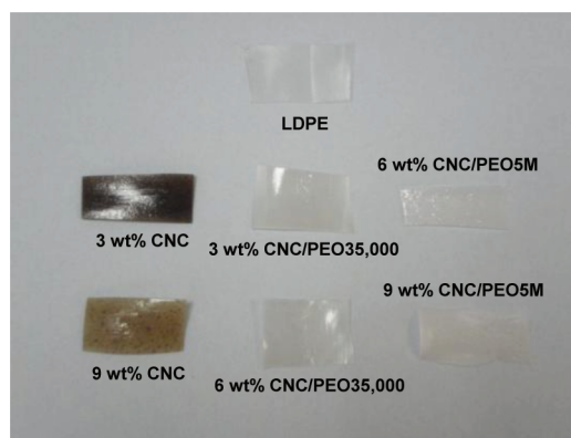
Figure 4. Pictures of the extruded films: unfilled polyethylene (LDPE) matrix and LDPE reinforced with neat CNC and PEO-adsorbed CNC.
